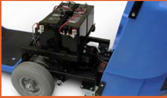
Flip-Up Rear Deck for Easy Service
