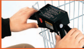
Thumb Lever Controls with Separate Forward/Reverse Switch Ideal for Mobility Impaired Riders
